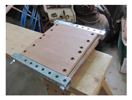
A metal frame is provided to simulate the presence of surrounding planking. The initial moisture content of the Wana was 13.3% and the AYC was 11.5%.
