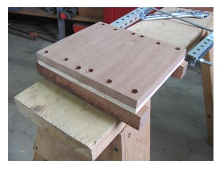
The picture above shows a sample of double planking with two 5/8" x 4" Wana outer planks on top of three 3/8" Alaskan Yellow Cedar inner planks, with Sikaflex 291 LOT between the two layers (about .6 mm; no primer). The planking is then screwed to two H. Mahogany frames.
