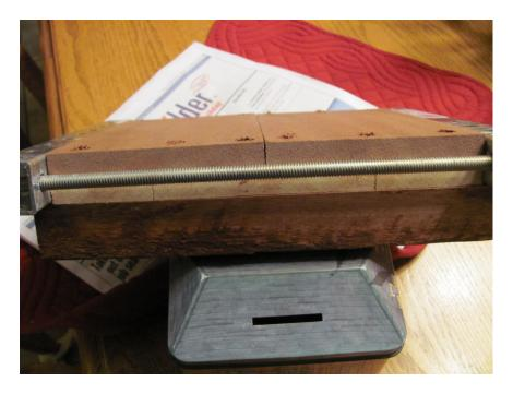
After 7 days of immersion, the sample was allowed to dry for 7 days at room temperature and low relative humidity. The picture above shows the sample after this drying period.
