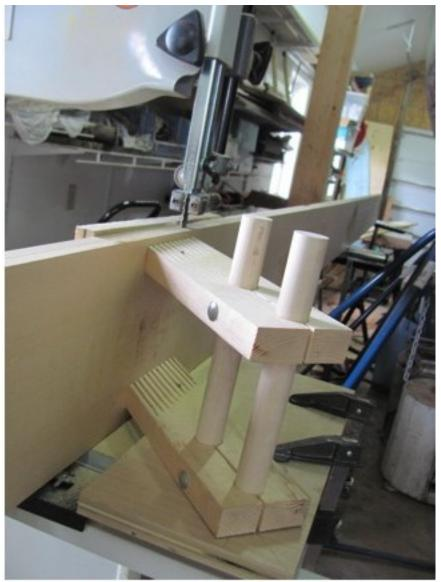
First I made an 8" high auxiliary fence that I bolted to the Wilton fence. I then free handed a piece of pine to determine how the blade (3/4" carbide) tracked. I then adjusted the fence angle parallel to the track line.
