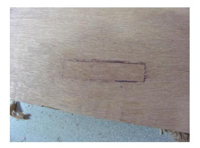
I used a marking knife to outline the hole and then used a mortising chisel to cut the hole. (bottom of hole cleaned out with small hand router.) I then sawed and planed a plug to fit. I suppose that fitting the ends as a scarf would be better structurally, but probably overkill for such a small repair.
