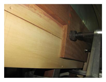
The first fit was a bit disappointing (more than .085" gap in one spot). But after just two cycles the maximum gap was less than .022".
