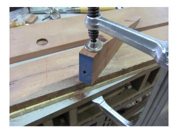
To make the guide, I insert a dowel into the hole and measure the angel (relative to the face of the plank) with a bevel gage. I also trace the angel that the bevel gage makes along the face of the plank. I then drill a hole in my guide matching the angel of my bevel gage. Then I align the guide along the tracing on the face of the plank. Then inserting the dowel into the guide, I slide the guide along the tracing until it enters the hole. I'm then ready to drill.
