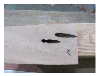
For these, I use a Dutchman repair; i.e., a rectangular plug much like a mortise and tenon joint.
