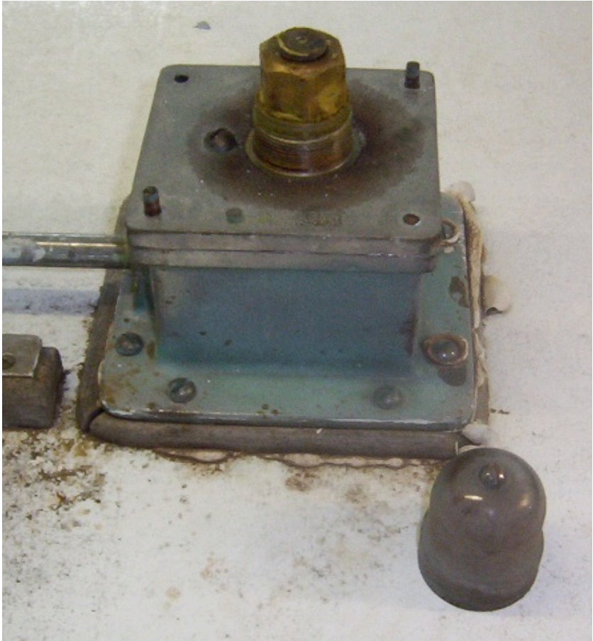
This pic shows a closeup of the gearbox with the cap removed, revealing a large bronze nut.
