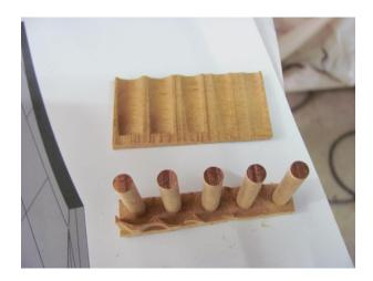
Finally, I separate each plug, leaving a plug with a little square top. This top makes it easier to hold the plug when applying the glue.
