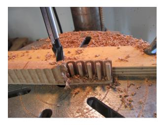
After making a row of plugs, I use a band saw to remove the row from the stock and again to separate the row of plugs from the straight edge.
