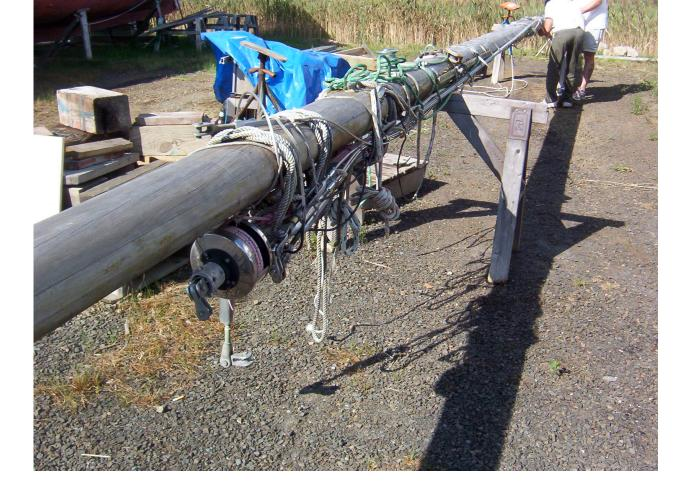
The mizzen boom is pristine. The main boom will have to be re-glued or replaced.
