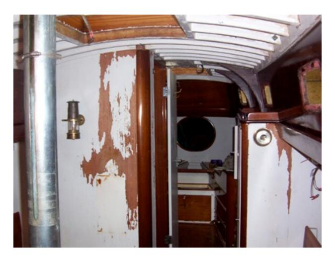
Main cabin looking aft. Galley sink above the engine compartment. Stove to the right (port) and ice box to starboard. The ice box was fitted with a cold plate; however, the compressor was found laying in the bilge. Evidently, the original engine was replaced but the compressor was never fitted to the new engine.
