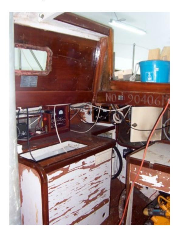
Kerosene stove on port side of galley. Bronze fuel storage behind the cabinets behind the stove. A manual priming pump below the stove on the right (not visible).
